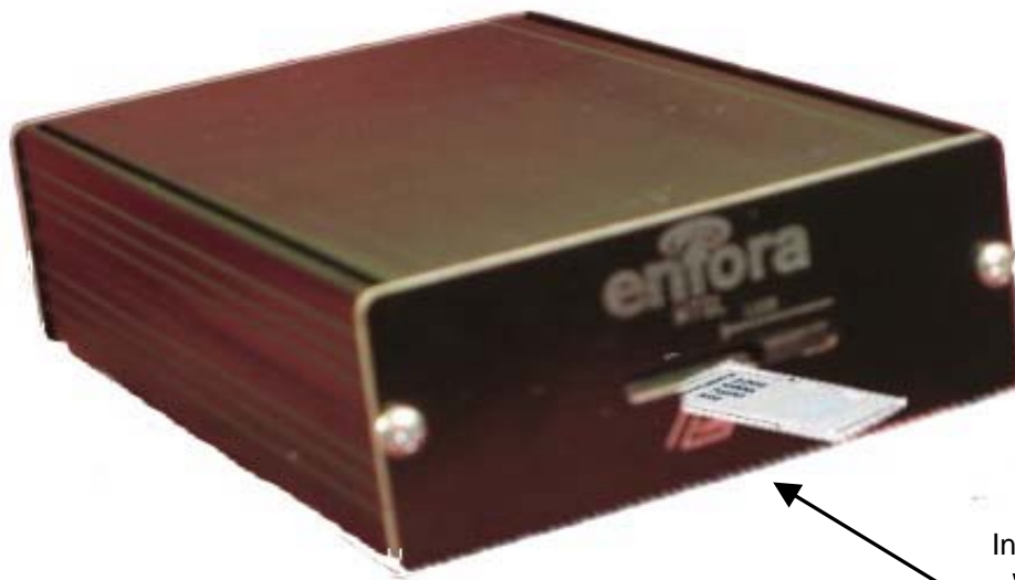
Figure 10 - Inserting a SIM
